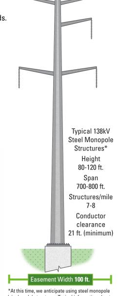
\*At this time, we anticipate using steel monopole (single pole) structures. Typical information about these types of structures is provided above. Note, this graphic is not to scale and the number of arms on a typical structure may vary depending on the final route.
