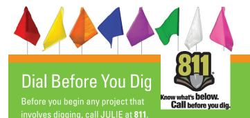
This will ensure that potentially hazardous underground public utilities are located and marked, so you can dig safely. The service is free, and it's the law.
