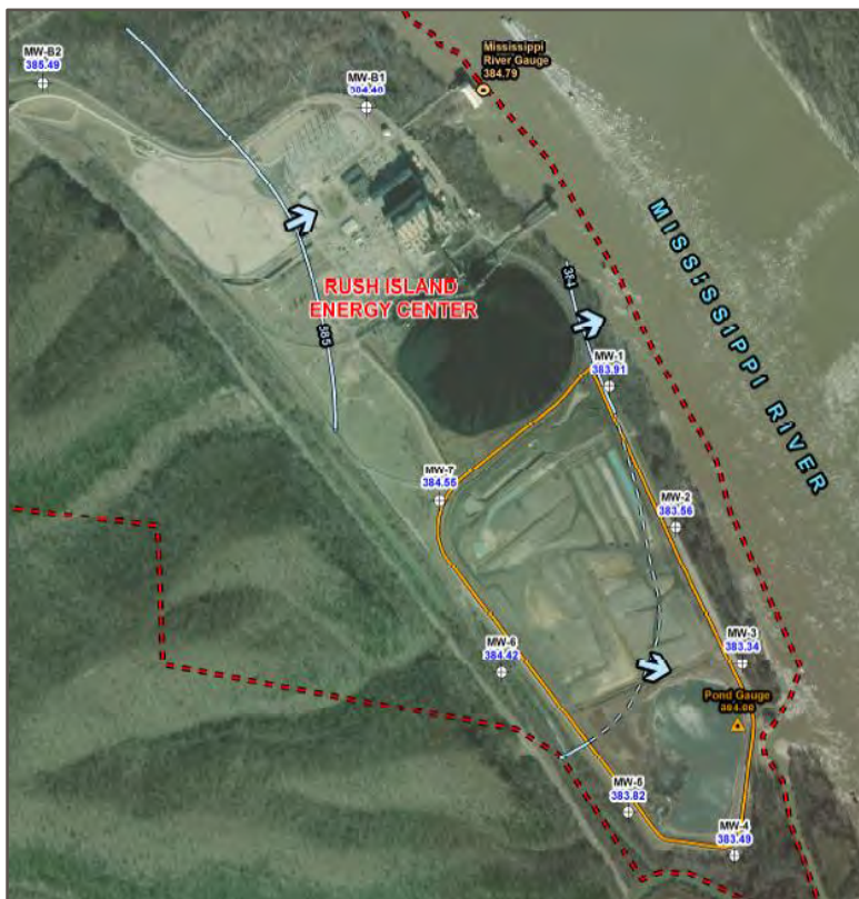
Groundwater Flow Map- November 1, 2018 Image from Figure C3, 2018 Annual Groundwater Monitoring and Corrective Action Report (Golder 2019)
