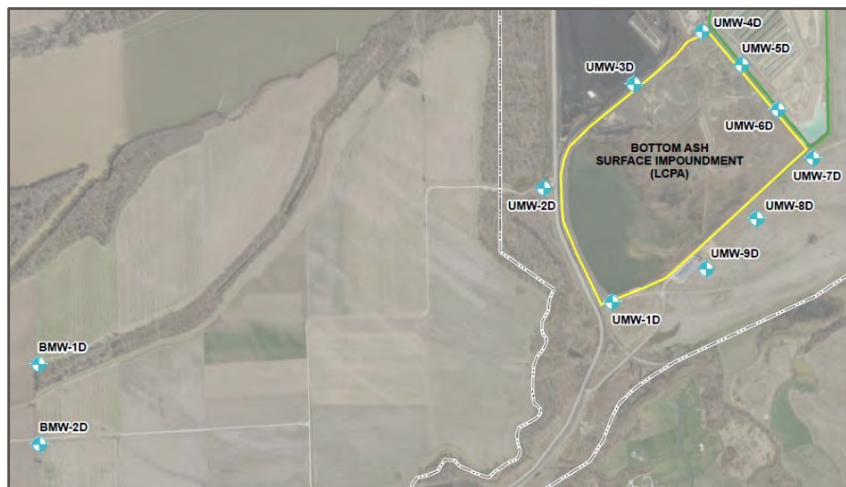
Groundwater Monitoring Well Locations
