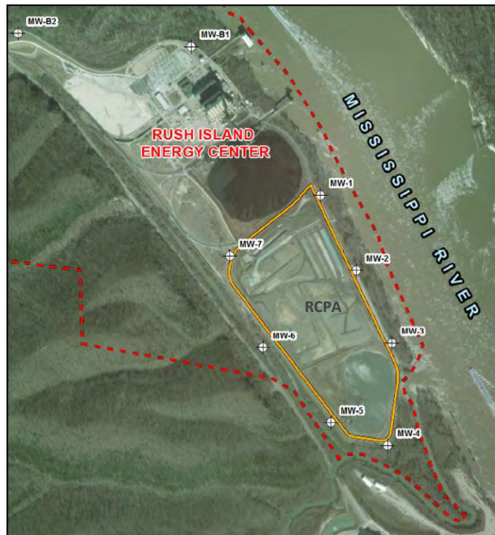
Groundwater Monitoring Well Locations Image from Figure 2, Groundwater Monitoring Plan (Golder 2017)
