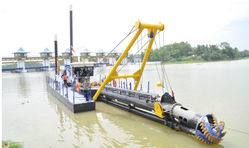
Figure 2 – Illustration of Cutter-Head Suction Dredge
