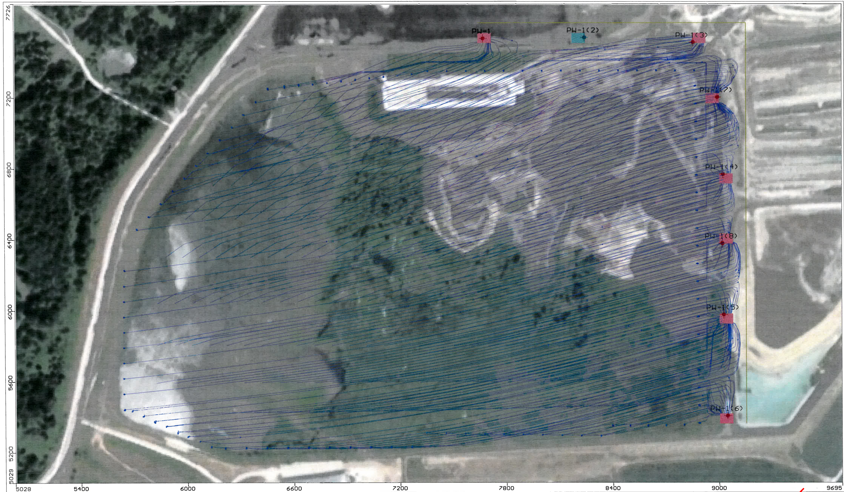
Appendix 6B-3: Flow Path Tracing from Bottom Ash Pond Hydraulic Control Via Pumping Wells, Barrier Wall to 407.5 feet elevation, and 10-7 Cap Wells Pumping at 20, 0, 10, 10, 15, 20, 15, and 10 GPM (Total Q = 100 GPM)
