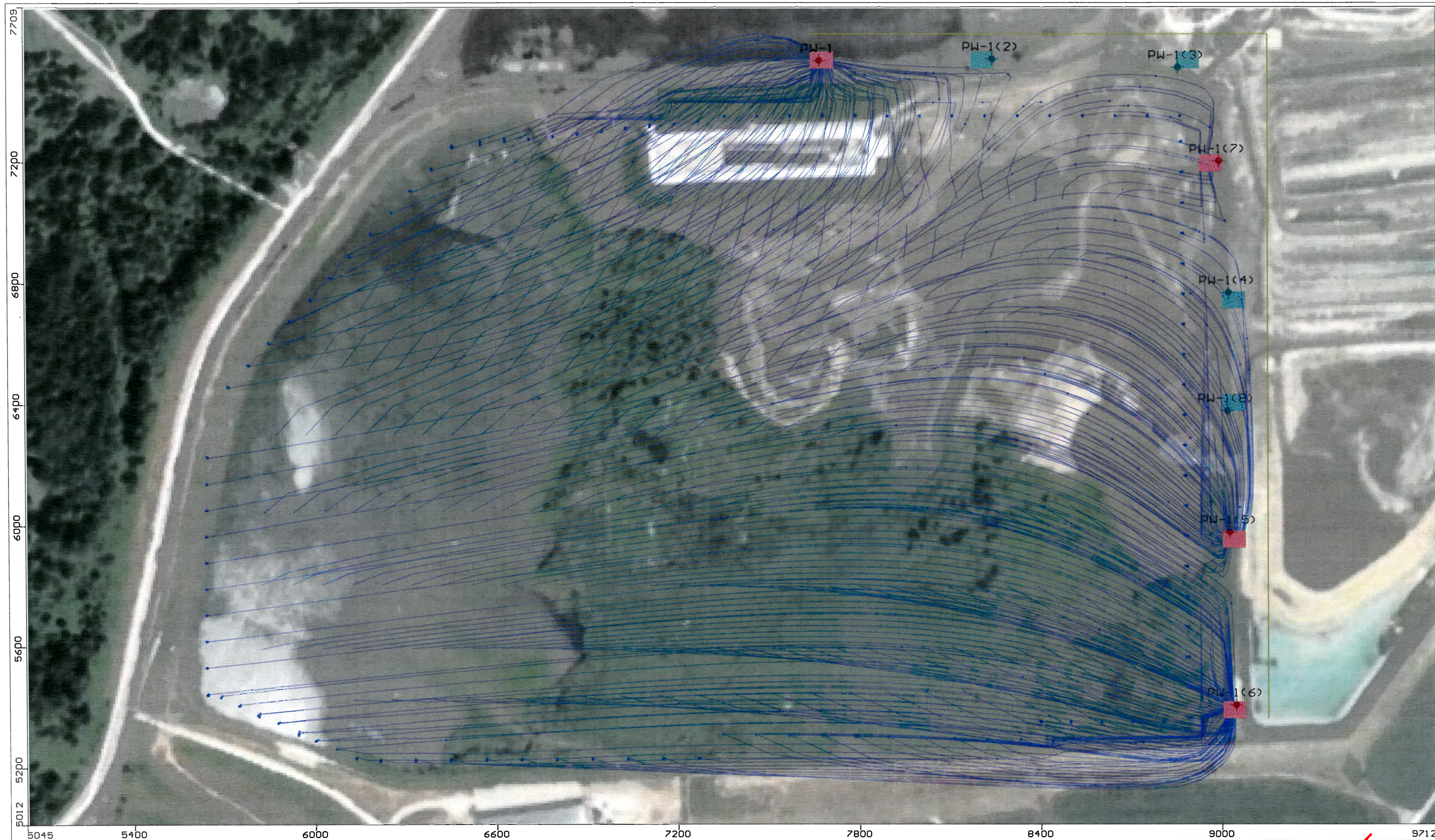
Appendix 6B-4: Flow Path Tracing from Bottom Ash Pond Hydraulic Control Via Pumping Wells, Barrier Wall to Bedrock, and 10-7 Cap Wells Pumping at 40, 0, 0, 0, 20, 50, 5, and 0 GPM (Total Q = 115 GPM)
