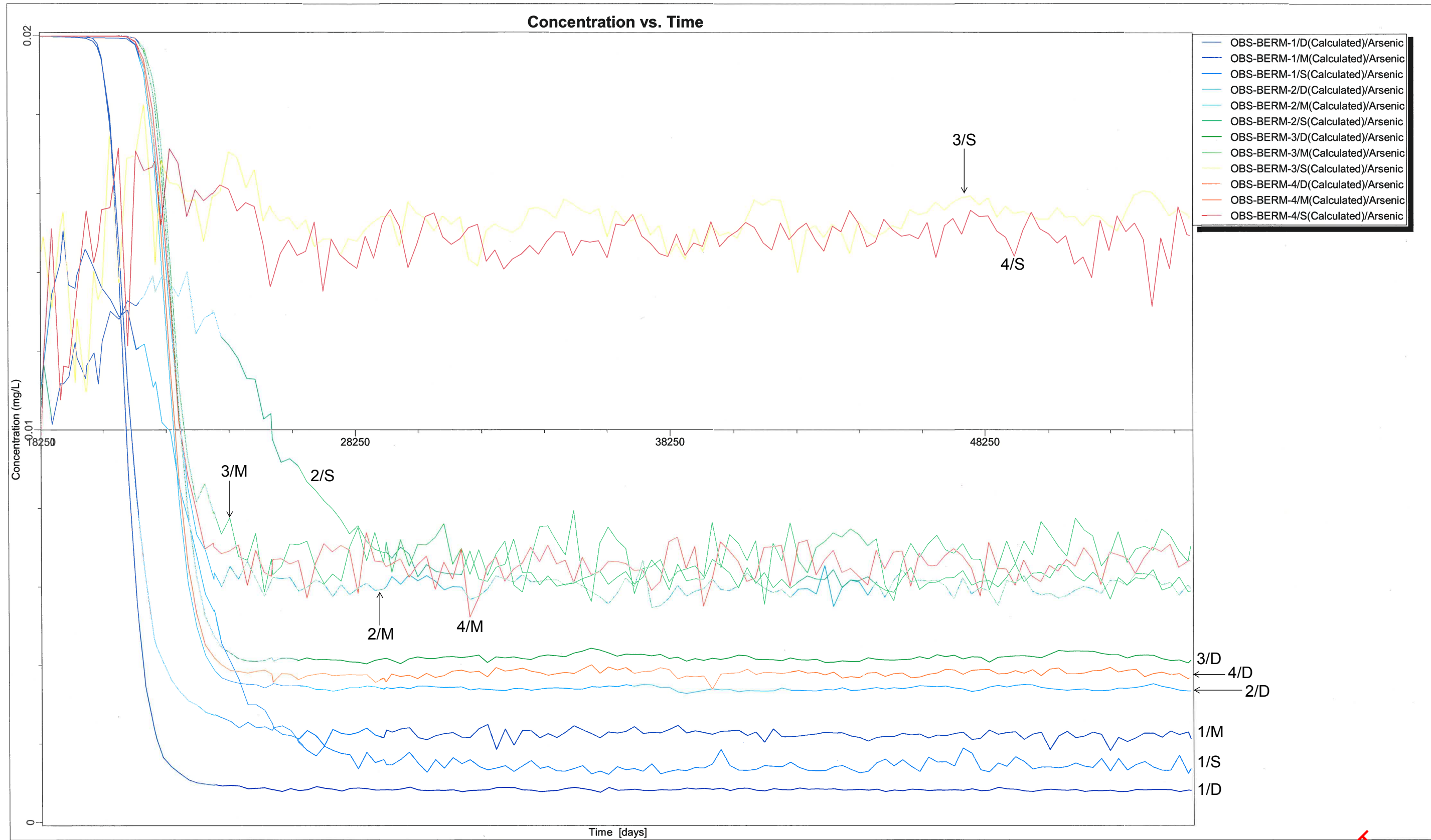
Appendix 5: Predicted Arsenic Concentration Time Series - Berm Observation Locations Simulated Source Concentration = 0.020 mg/L 10-7 Cap, No Hydraulic Controls
