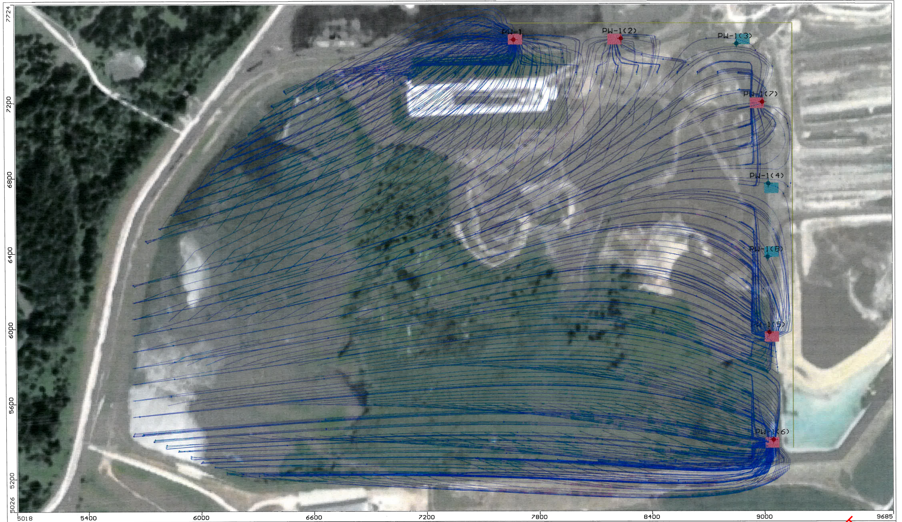
Appendix 6A-4: Flow Path Tracing from Bottom Ash Pond Hydraulic Control Via Pumping Wells, Barrier Wall to Bedrock, and No Cap Wells Pumping at 60, 15, 0, 0, 40, 70, 20, and 0 GPM (Total Q = 205 GPM)
