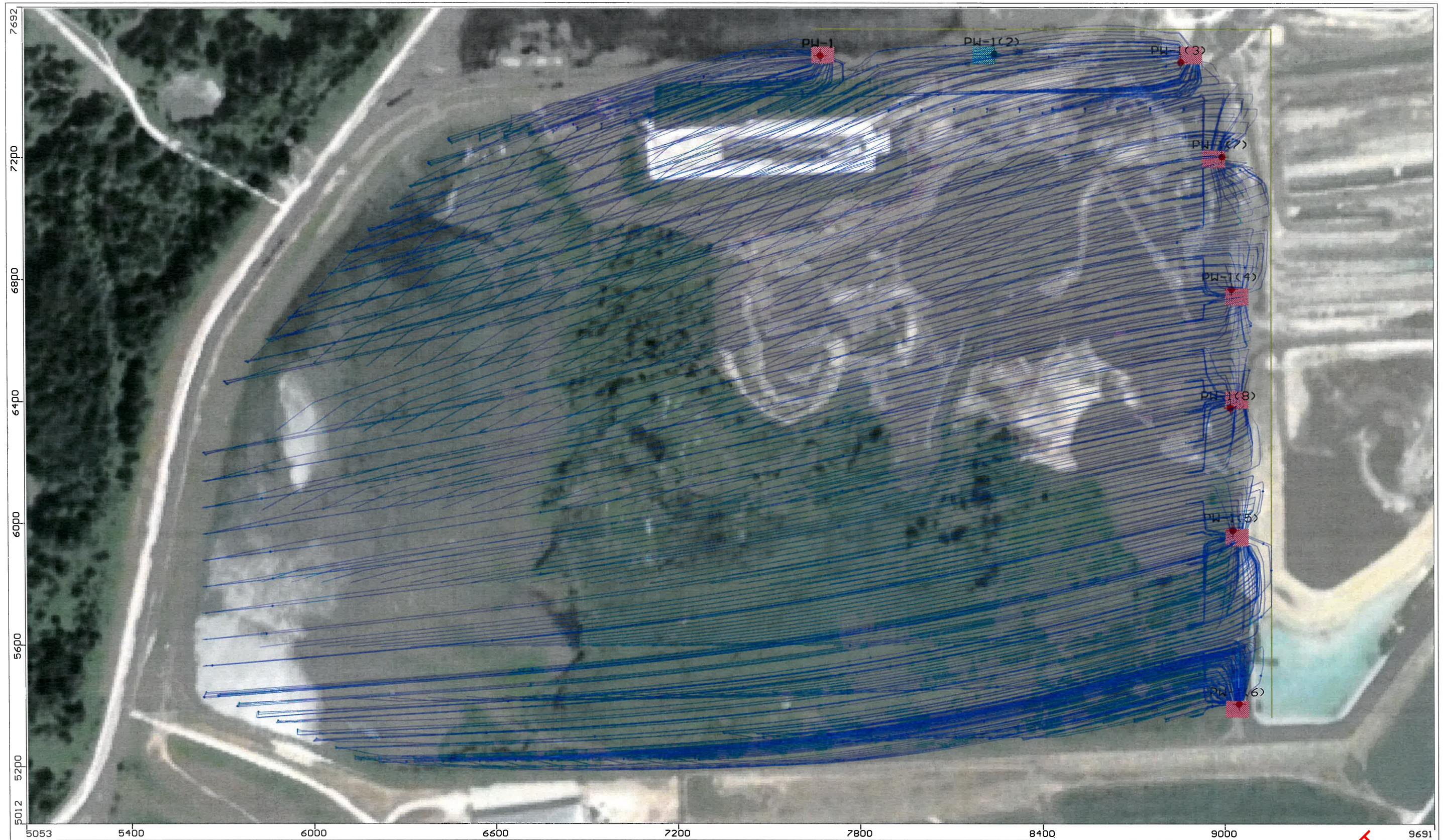
Appendix 6A-3: Flow Path Tracing from Bottom Ash Pond Hydraulic Control Via Pumping Wells, Barrier Wall to 407.5 feet elevation, and No Cap Wells Pumping at 15, 0, 25, 25, 35, 40, 25, and 30 GPM (Total Q = 195 GPM)
