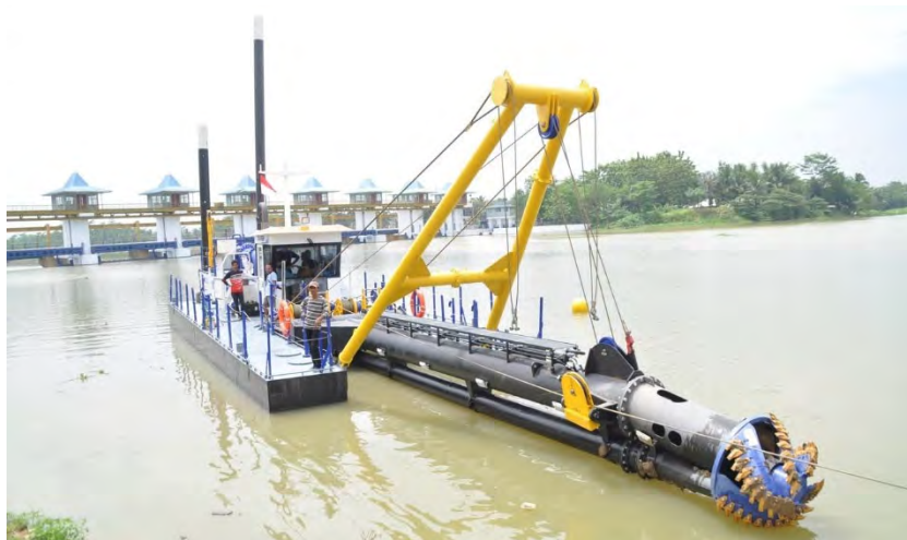
Figure 2 – Illustration of Cutter-Head Suction Dredge
