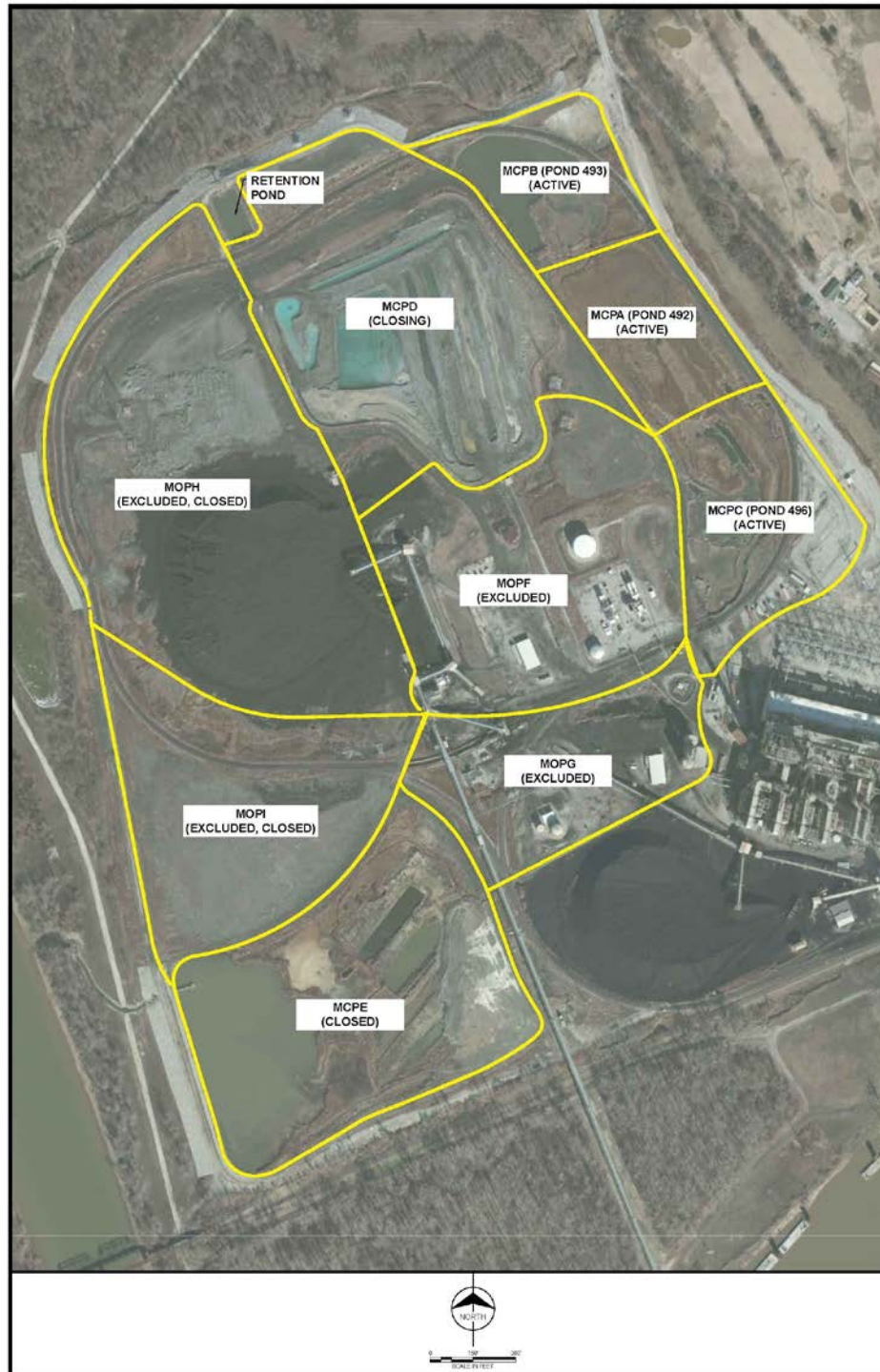
FIGURE 2 – MEC SURFACE IMPOUNDMENTS
