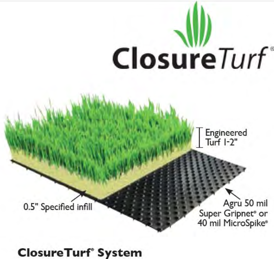
Exhibit 2 – Example Alternative Synthetic Alternative Final Cover System (From Agru America Closure Solutions Brochure)
