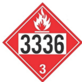
Figure 1: DOT HAZMAT Placard for bulk odorant loads
