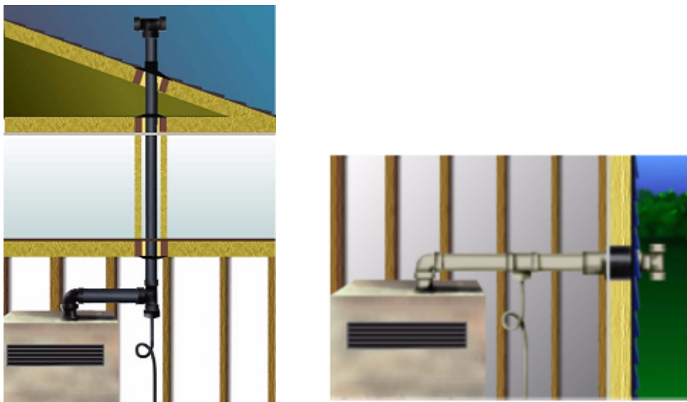
Figure 2: Examples of Recalled Plastic Vent Pipe Systems
