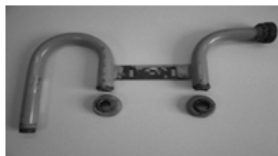
Figure 2: RW Lyall 10LT Corroded Meter Spud Welds
