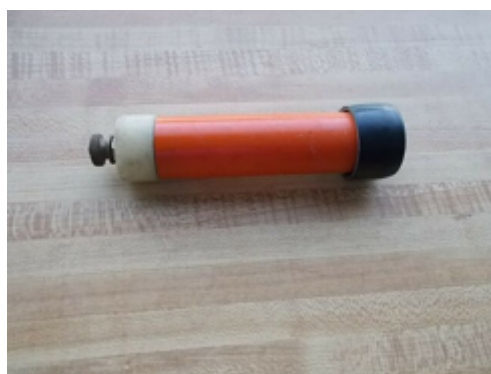
Figure 2 Copper-copper Sulfate reference cell
