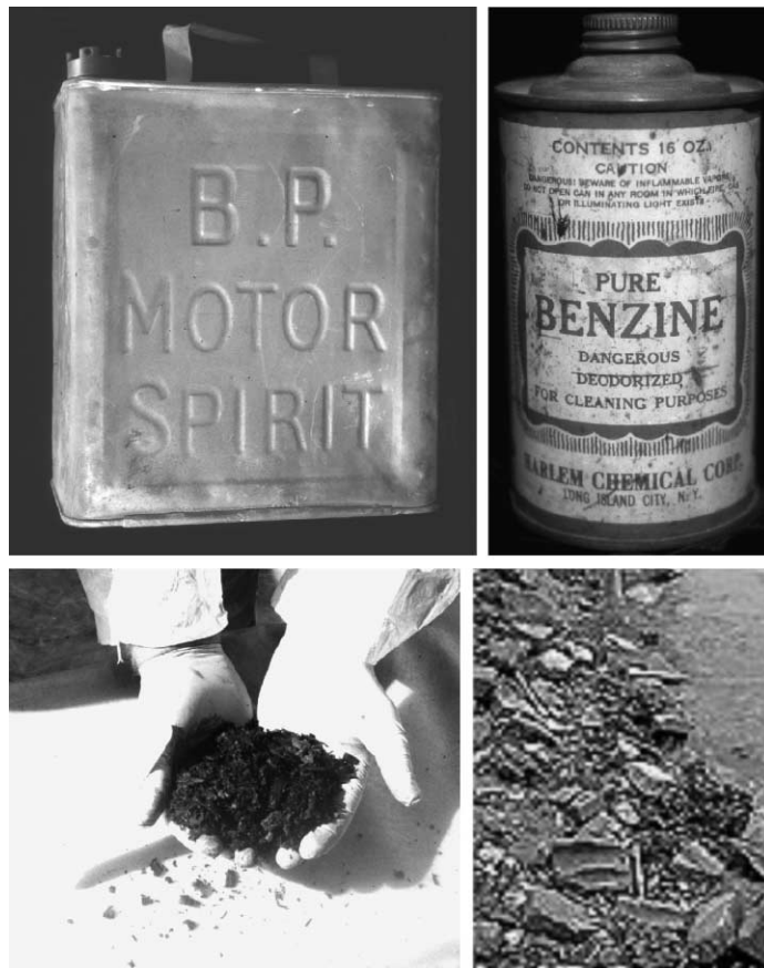
Fig. 5. Some outstanding gas works residuals. (5L) Motor spirit (a.k.a. Benzol) was the forerunner of our gasoline and benzine was a distilled derivative of the benzol. Today, these two light nonaqueous-phase liquids (LAPLs) are commonly found as groundwater contaminants, though more often not as free phase (from the Author's collection). (5L) The motor spirit can is British and holds one imperial gallon (both are from the author's collection). (5LL) Freshly excavated box-waste wood chips from the gas works dump at Sacramento FMGP no. 2, California (photographed by the author, 1999). (5RR) Typical appearance of the gas works dump at creek or riverside. This is at Manistee, MI (photographed by the author, 2001).
