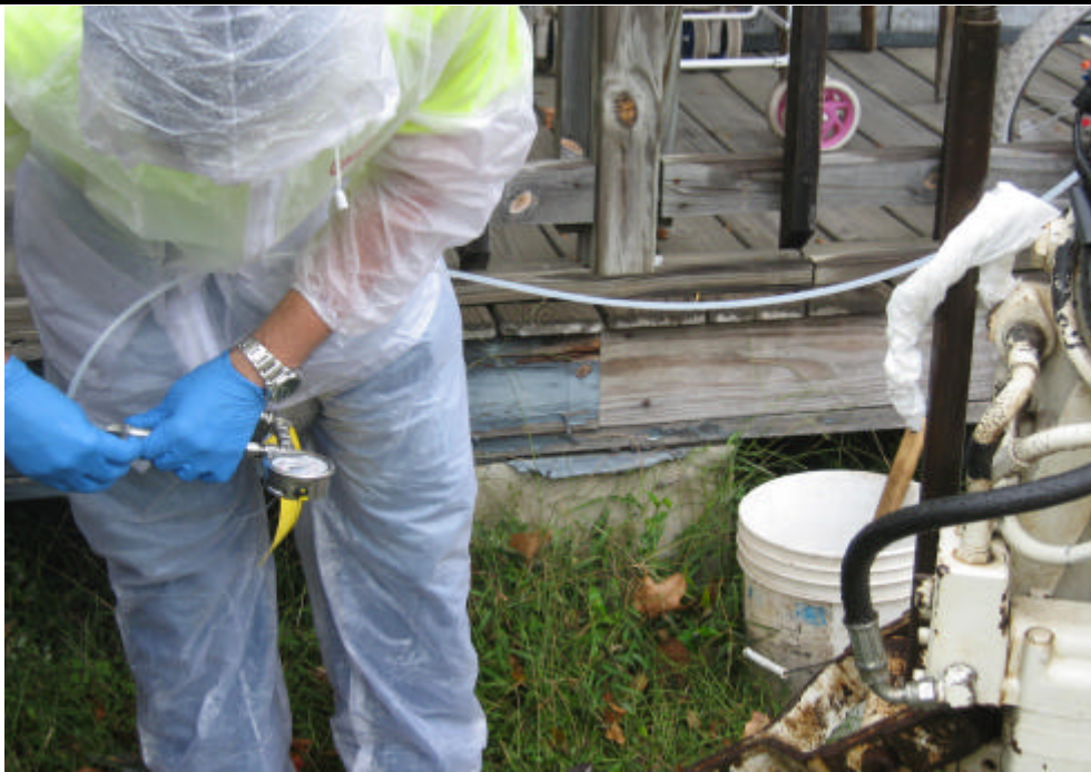
PHOTO 7: Attaching 1-Liter SUMMA canister at VP412EHill-3 location. Note white paper towels with leak detection compound wrapped around equipment.
